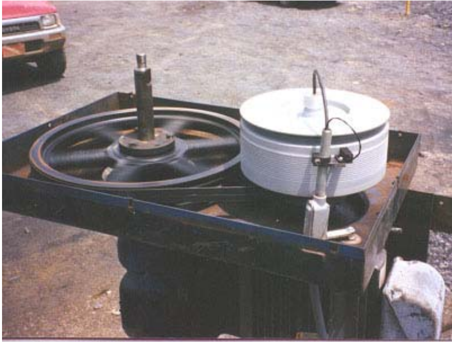
Field retrofit shown with cover removed for illustration purposes. The drive simply replaces the original motor pulley
